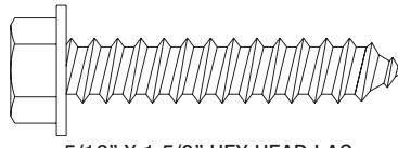
5/16" X 1 5/8" HEX HEAD LAG SCREWS (AS REQUIRED)
